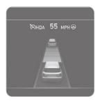
NOTE: If the engine is turned off then on again, the function maintains the last setting. Highway Driving Assist helps maintain a set distance and speed from the vehicle ahead and helps center the vehicle in the lane, and automatically adjusts the vehicle speed to the speed limit while driving on the highway.
